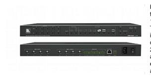
Kramer's VSM 4x4X is a 4X4 seamless matrix switcher that can also be used as a video wall driver (2X2 or 1X4), a quad-viewer, or a 4 picture multi-viewer. The unit allows instantaneous switching between inputs (that is, with a clean, frame-to-frame video cut). The VSM 4x4X supports HDMI 2.0 and HDCP 2.2, with resolutions up to 4K60 4:4:4, per-port HDCP and EDID settings, passing of 4 channels of embedded audio, and analog stereo de-embedded audio for each of the 4 outputs
